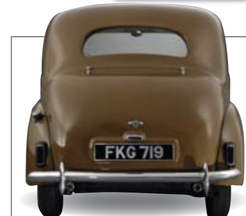
REAR This Barker-bodied car features a more modern, curvy-booted rear end than the Briggs version.
